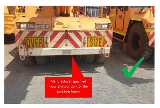
A recent crane incident resulted in a spreader beam dislodging from the manufacturer specified mounting point of a 25T Franna crane because the safety locking pins failed – The pins being used at the time were not the manufacturer approved pins
