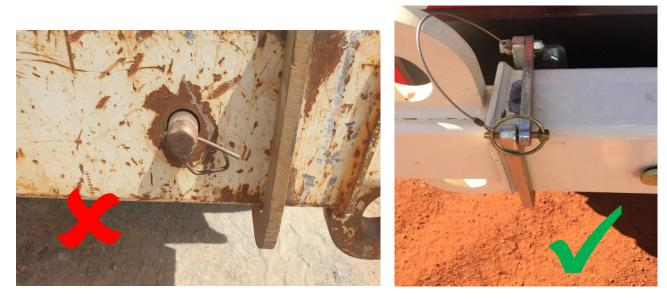
Photo on the left is an example of the wrong safety locking pin - photo on the right is the correct manufacturer specified linch pin for locking the spreader bar into place
