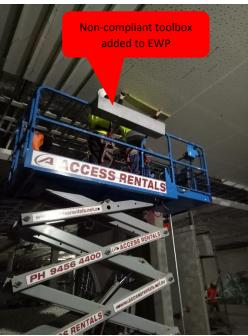
Elevated Work Platforms (EWPs) have been designed for a specific purpose. Adding, altering, changing or adjusting the EWP in any way, shape or form could be in breach of the design and manufacturing specifications, and could result in disastrous and devastating effects on the health and safety of all workers who work in, with and around these machines.
