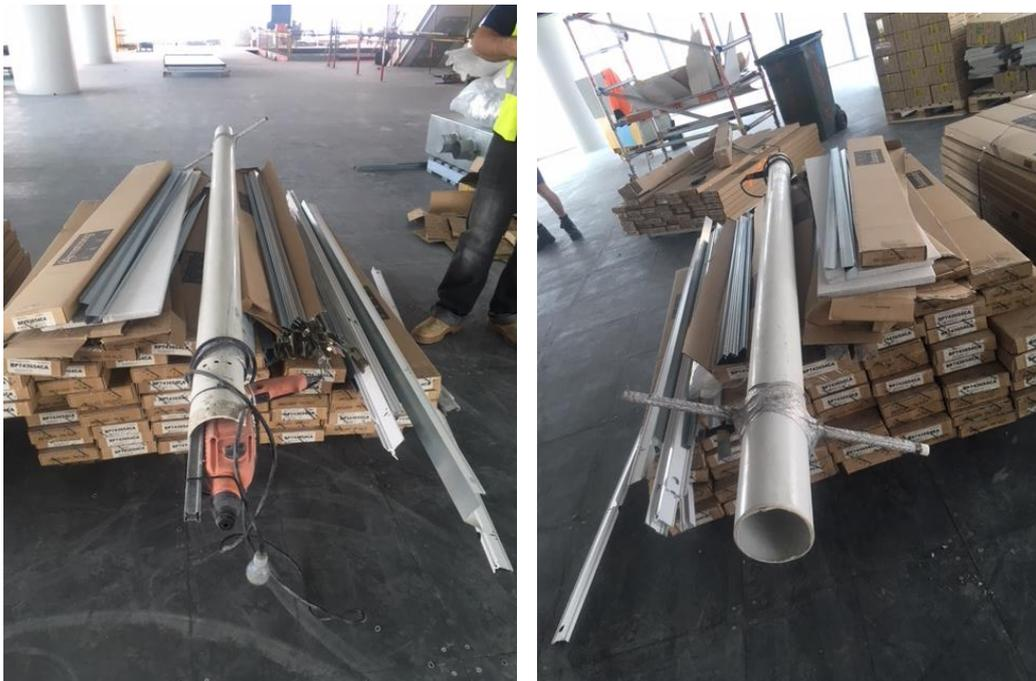
**Question:** Multiplex accepted this modified drill being used to reach an area where holes had to be drilled in a high location into the underside of a concrete floor slab from the level below. What's so hard about providing a work platform so that the job can be done using a drill in the way it was designed and intended to be used?
